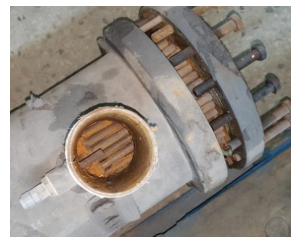
Disconnect to see tube diameter and pitch
